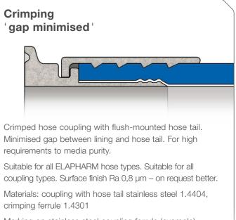
Marking on stainless steel coupling ferrule (example): ELAFLEX · Type · DIN · DN · PTFE · Serial Number · Month.Year · PT (bar)
