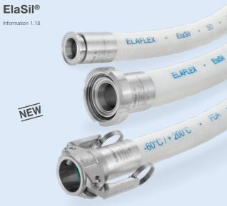
Silicone hose for high media purity requirements with smooth lining of platinum-cured, translucent, phtalate-free silicone. Highly flexiible, kink and vacuum resistant, large temperature range -60°C up to +200°C (depending on medium). Conform to FDA, USP Class VI and 3-A Sanitary Standard, suitable e.g. for cosmetics, pharmaceuticals and foodstuffs. Steaming out for cleaning and sterilisation possible, autoclavable.
