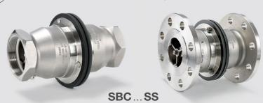
Passive safety: SBC Safety Break Couplings (Emergency Break-Away Couplings) are used within hose assembly lines and loading arm systems. They serve to protect against excessive pull forces. Modern construction, low pressure drop. For loading and unloading road and rail tankers, ships; also suitable for offshore use.
